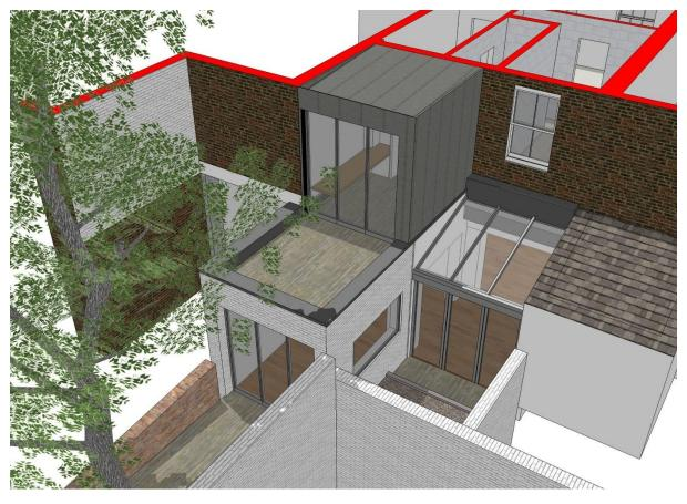
Design concept image showing semi-aerial view of proposed first floor metal clad extension, aligned with rear building line to adjoining lower terrace, and new glazing to rear offshoot elevation.
