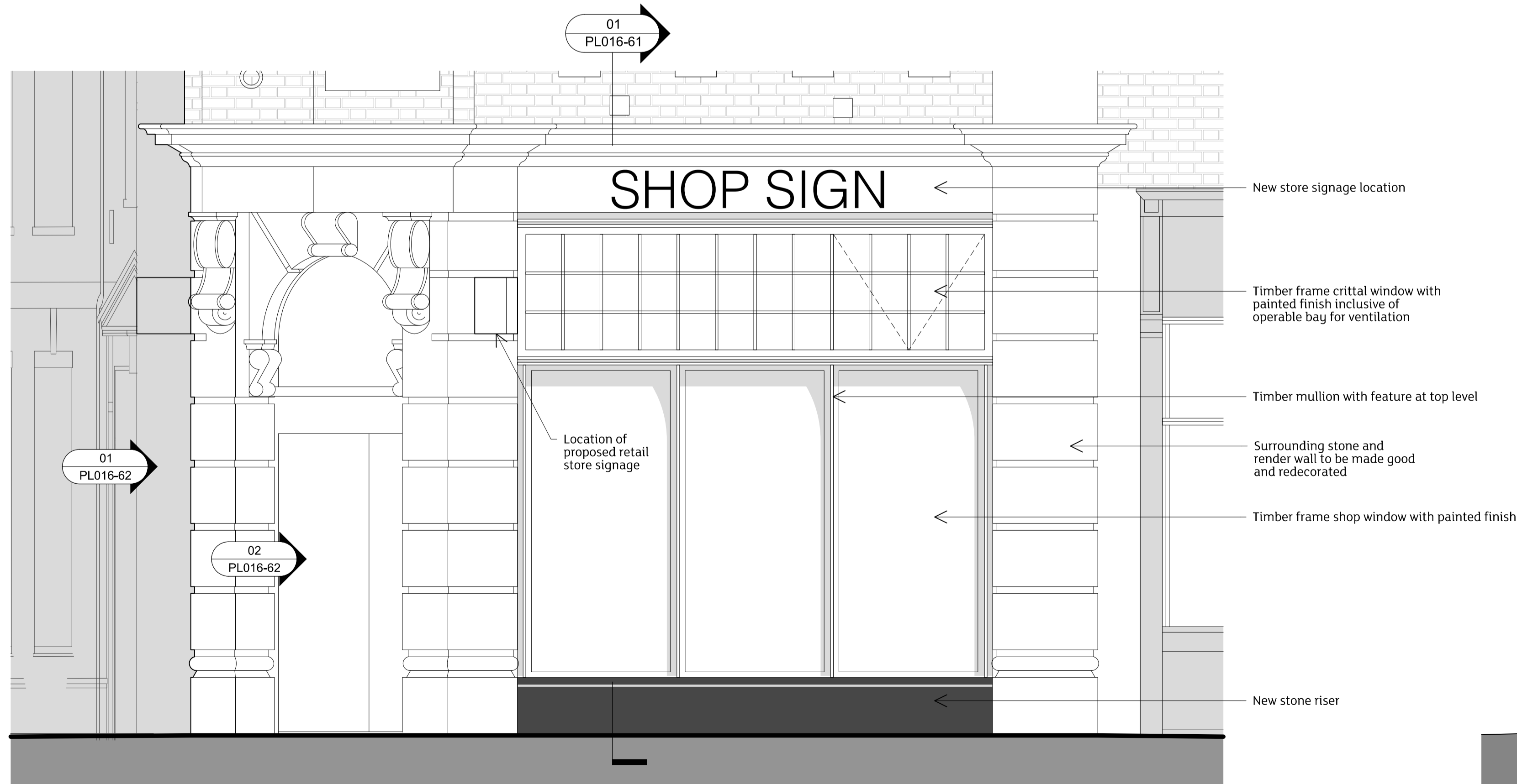
03 28 Denmark Street Proposed East Elevation 1:25
