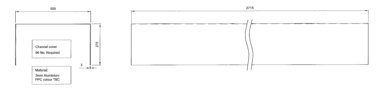
Fixing angle 96 No. Required Material: 1.5mm Aluminium 2715 PPC colour TBC
