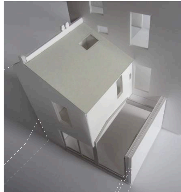
Aerial view of side extension and new roof light in sloping roof
