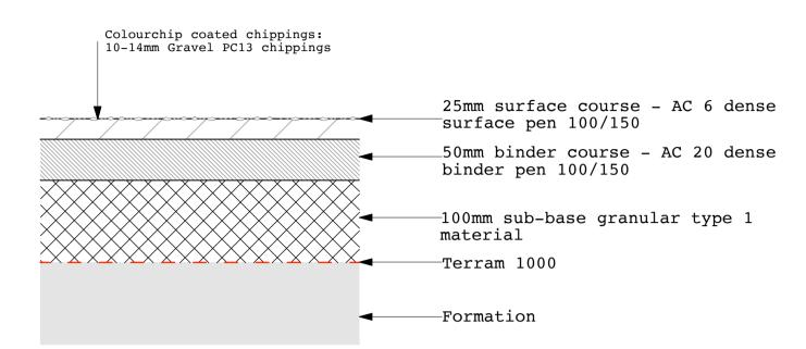
COLOURCHIP COATED CHIPPINGS: to be spread evenly over surface and rolled into hot ashphalt at time of laying.
