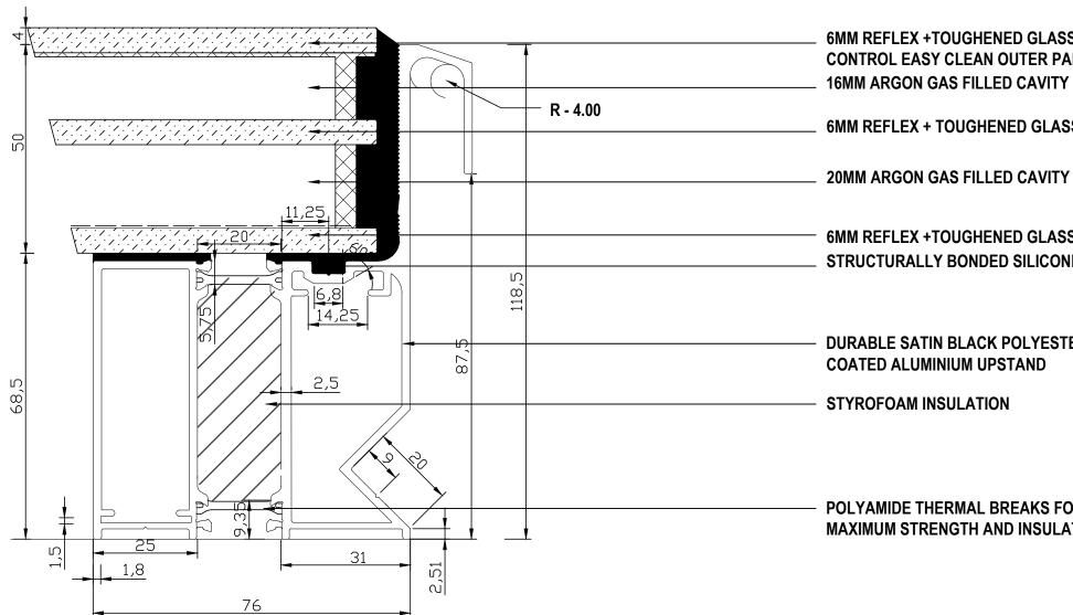
6MM REFLEX +TOUGHENED GLASS SOLAR **CONTROL EASY CLEAN OUTER PANE 16MM ARGON GAS FILLED CAVITY**
