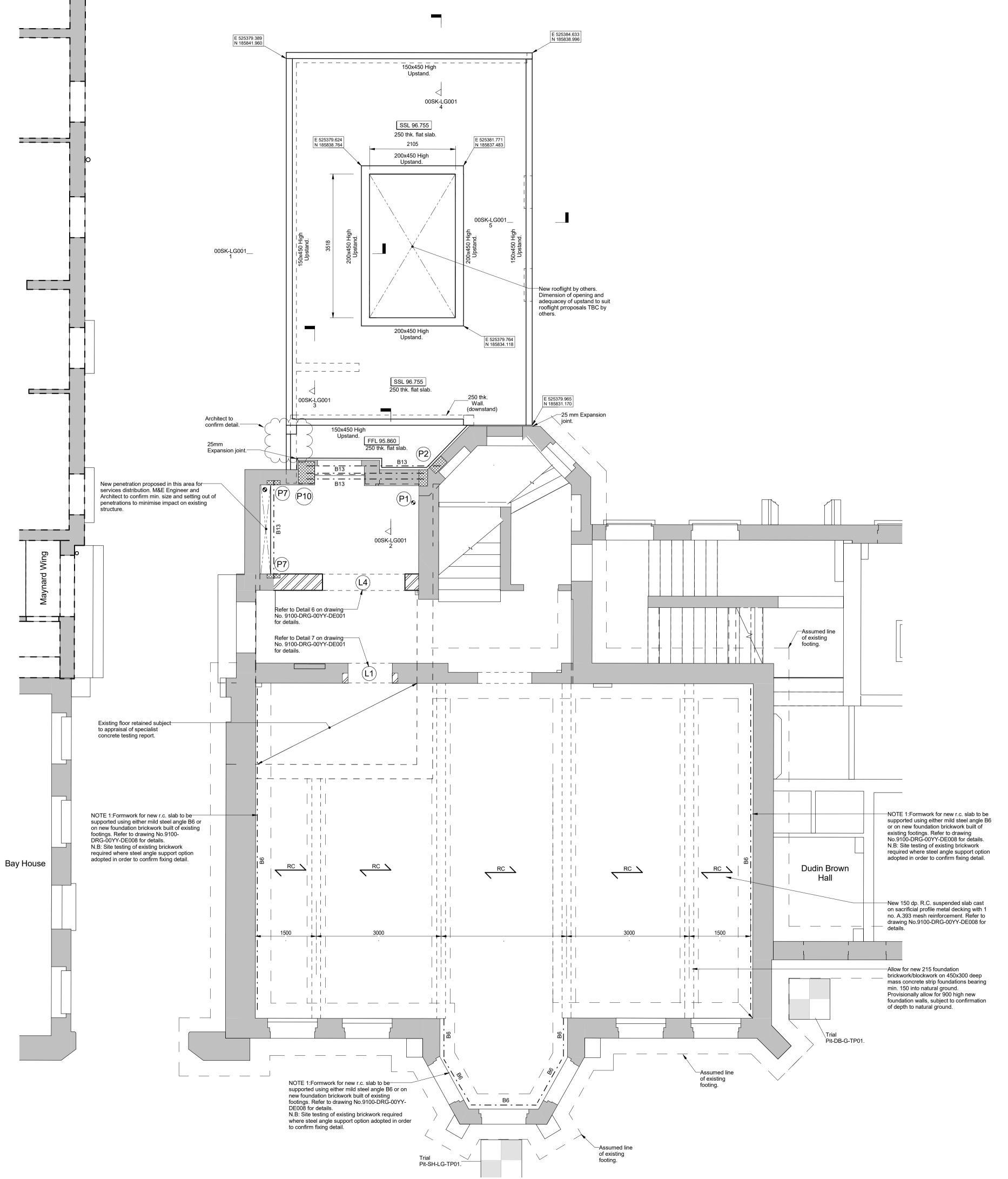
NOTE PROVISIONAL REPAIR ALLOWANCES SHOWN ON THIS DRAWING WILL BE CONFIRMED FOLLOWING STRIP OUT OF EXISTING FLOOR AND WALL FINISHES AND FOLLOWING ADDITIONAL OPENING UP WORKS. ENGINEER TO INSPECT EACH AREA IN TURN AND CONFIRM EXTENT OF REPAIRS REQUIRED.
