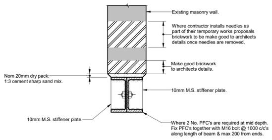
**Section 2-2: New 'PFC' Beamed Opening In Load Bearing Wall**
