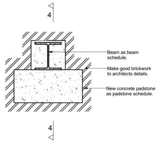
**Detail 3: Beam Support Detail: Type A**
