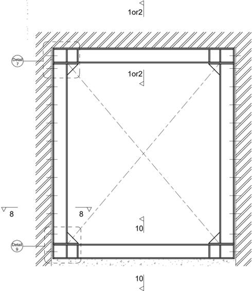
**Detail 6: Elevation on Generic Steel Box Frame**
