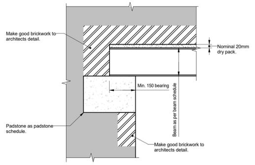
**Detail 5: Beam Support Detail: Type B**
