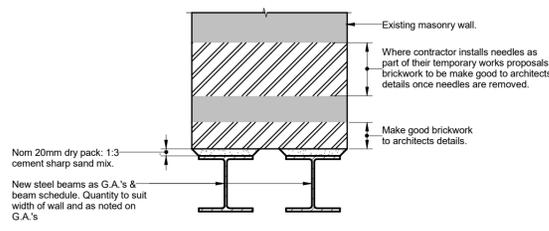
**Detail 1: New Steel Beamed Opening in Load Bearing Wall**
