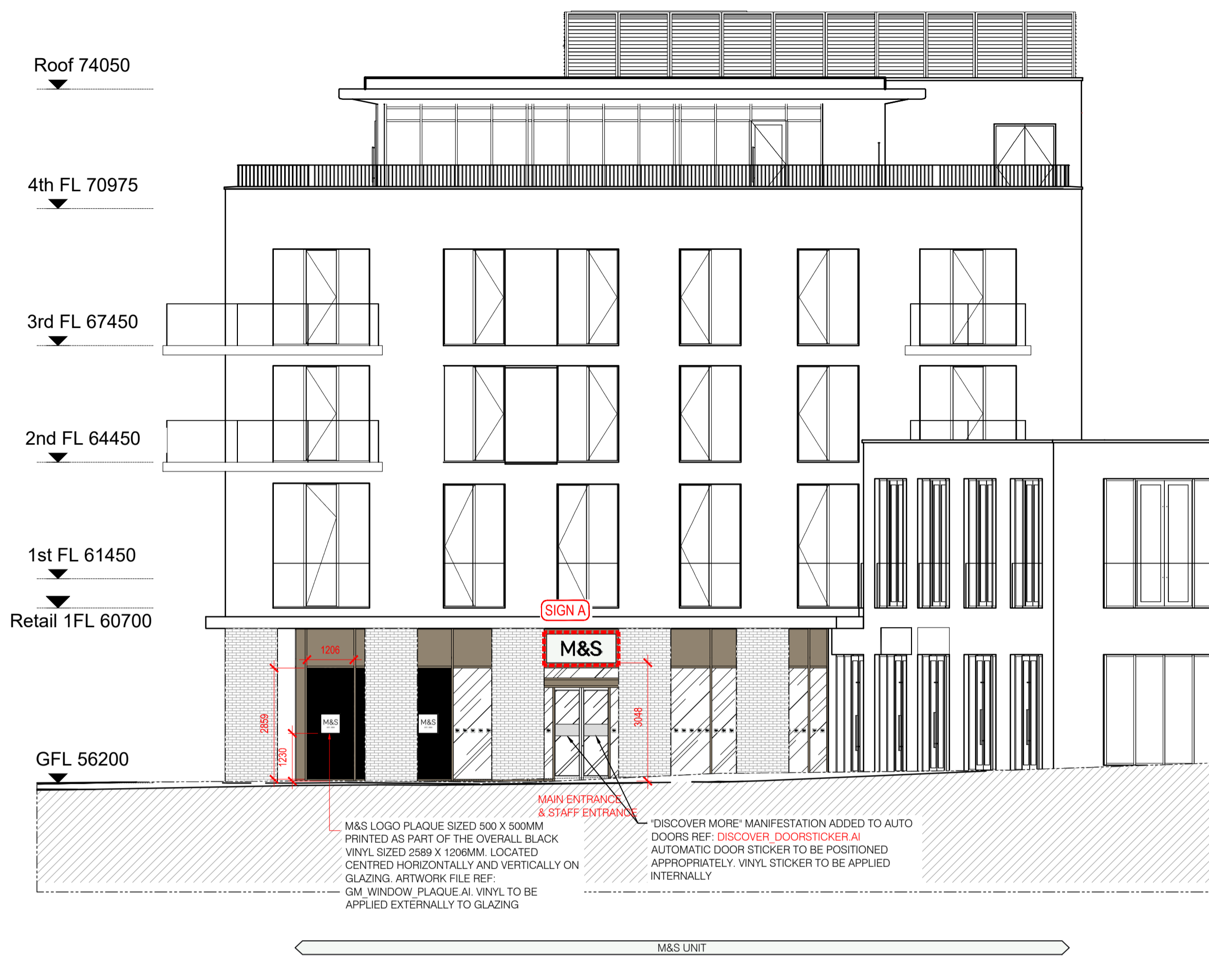
01 PROPOSED EAST ELEVATION 451 1:100 (WITH BRICKWORK)
