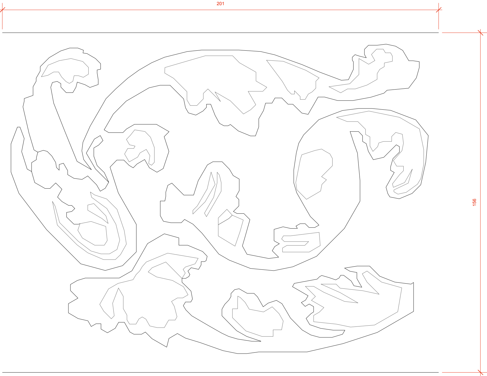
1 DETAIL OF PROPOSED NEW PLASTER CORNICE THROUGHOUT GROUND FLOOR Scale: Actual Size
