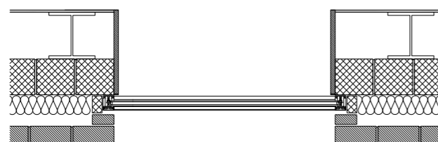
Roof - Window Reveal Detail - Plan
