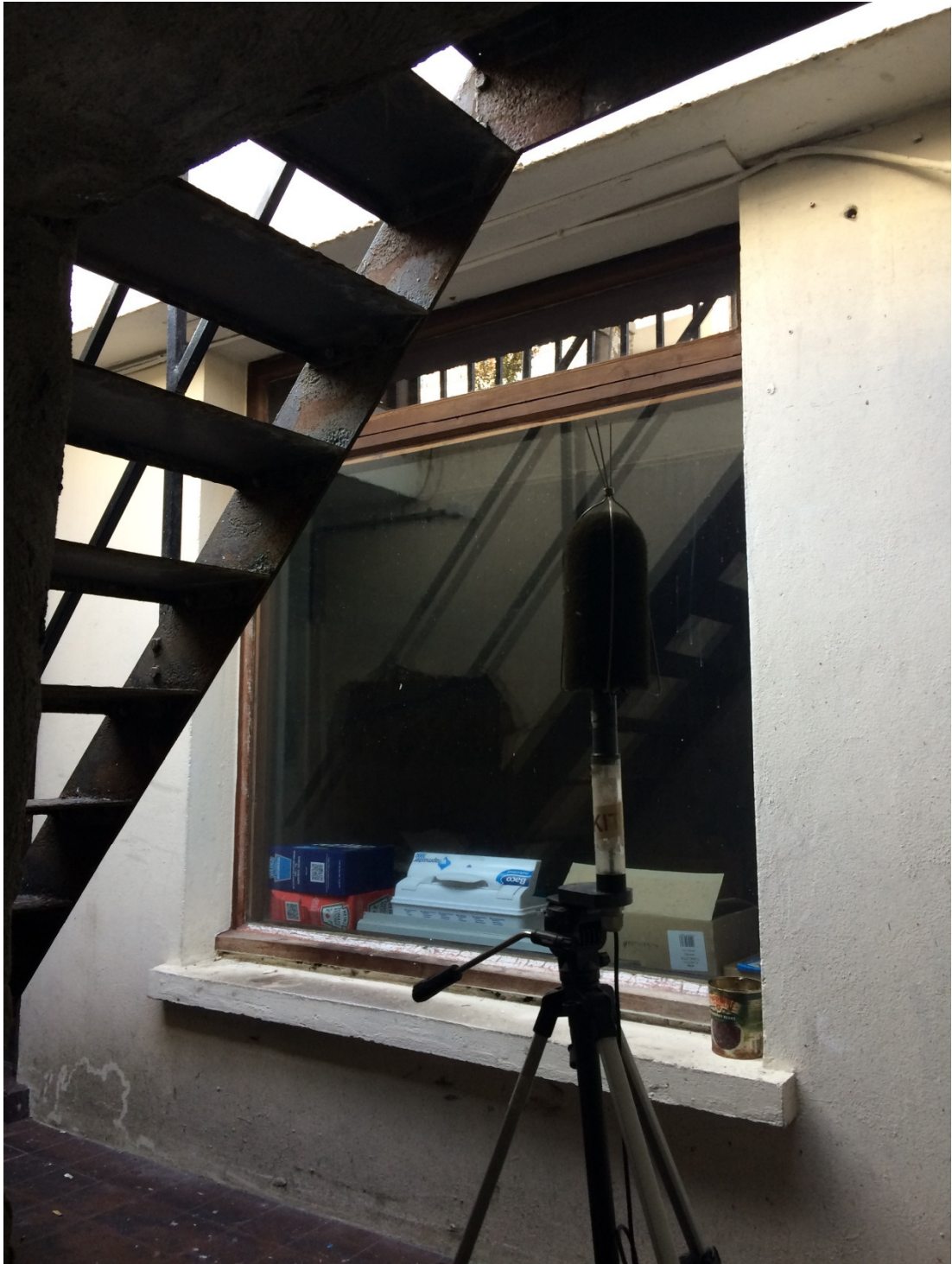
Figure A1.1: Noise Monitor in Front Lightwell
