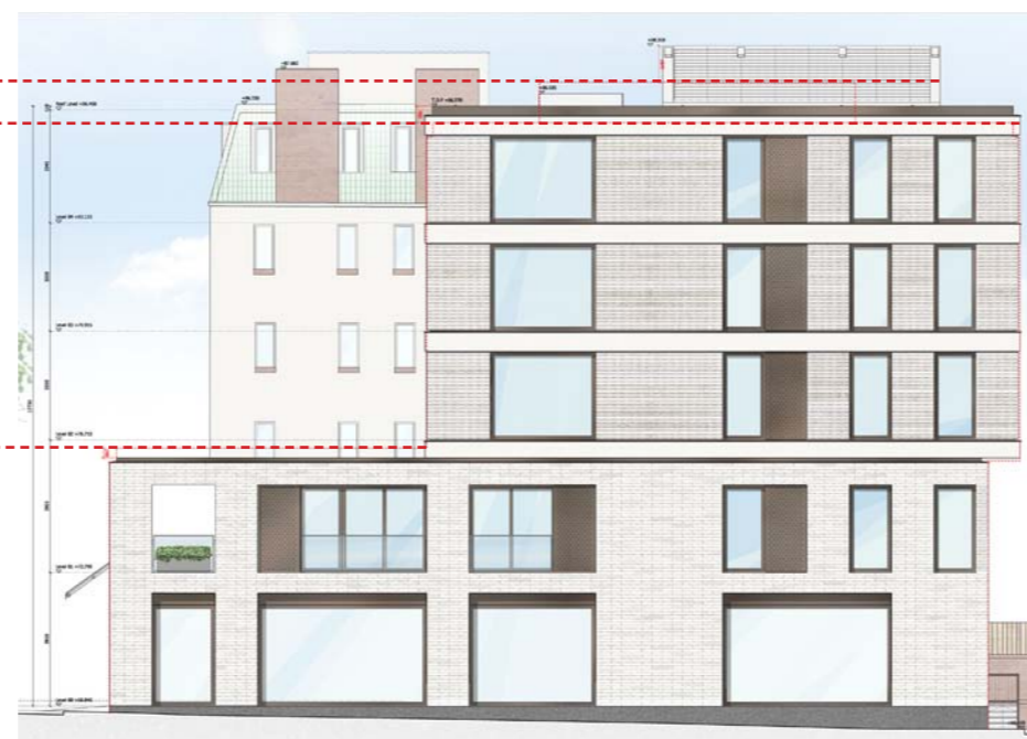
Proposed SE (side) Elevation - front coping reduced and top section raised so that a shadow gaps is created consistently along the building.
