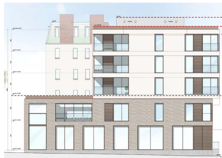
Consented SE (side) Elevation - front coping runs into base of second floor
