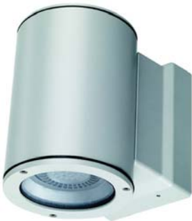
ITEM 10 (Qty 3) Narrow beam Mono Light 175 LED emission wall mounted luminaire. Die-cast aluminium construction finished in powder coated silver. Tempered safety glass lamp cover to single emmission
