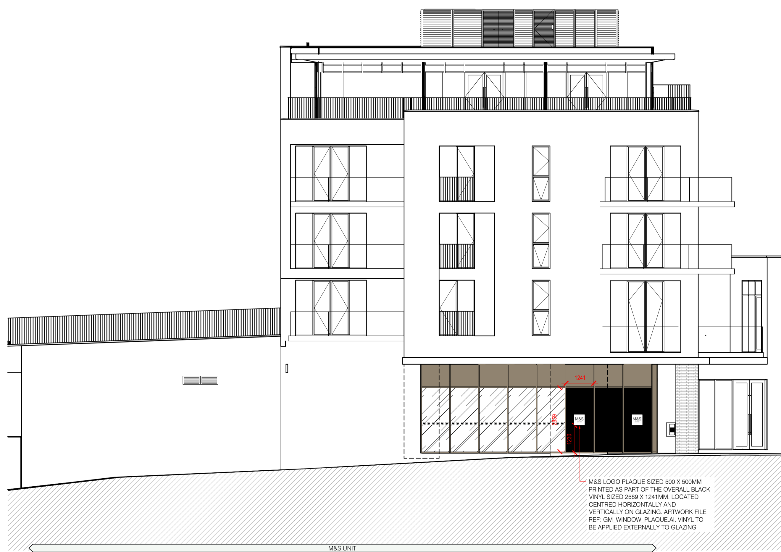
02 PROPOSED SOUTH ELEVATION (WITHOUT BRICKWORK) 452 1:100 SHOPFRONT GLAZING
