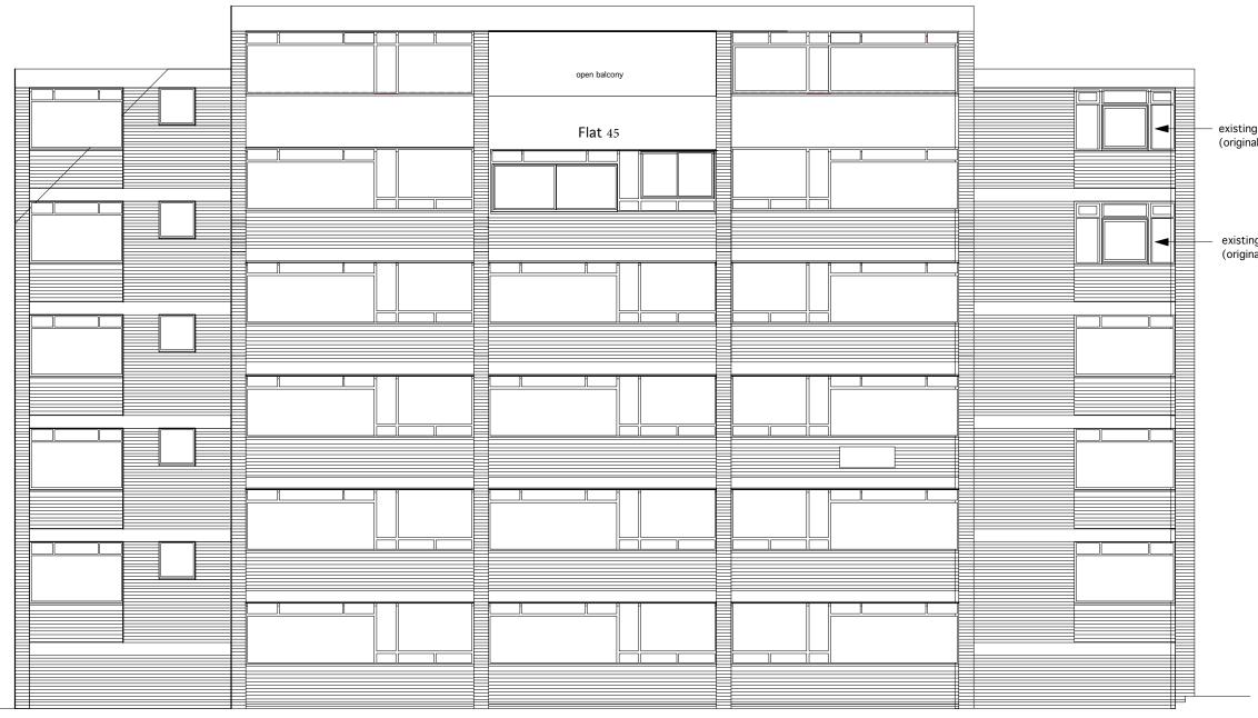
Existing Materials: Brick cross walls and brick panels between exposed floor concrete facias Concrete roof facias Concrete spandrel panels at 5th floor Tile hung spandrels ground to fourth Windows: brown painted hardwood single glazed
