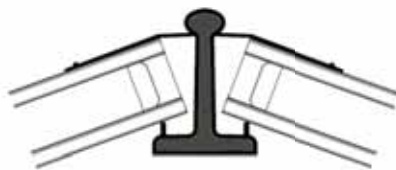
Heritage LC7 DG type lead covered steel hip glazing bar - double glazed
