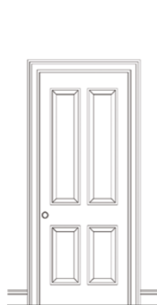
DOOR ALL LOWER GROUND FLOOR DOOR AND ARCHITRAVE PAINTED
