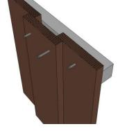
Shiplap cladding should be installed with one screw/nail for each stud. Secure the screw/nail approx. 1/3 in from the edge of the board, so that the pressure on the overlapping boards is a great as possible.
