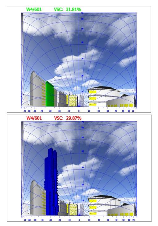
The point of reference is the same as for the skylight indicator, at the centre of the outward window face. Effectively a snap shot is taken from that point of the sky in front of the window, before and after the obstruction is put in place together with all the relevant obstructions to it, i.e. the buildings.
