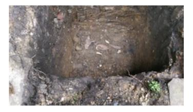
4.3.3 As is evident from the site photographs very limited root activity has been encountered during the hand dug excavations for this trial pit. As with trial pits 1 & 2, the face of within the trial pit closest to the Hawthorn tree, T3, shows minimal fibrous root growth with no larger anchorage tree roots. Some fibrous root activity at ground level as shown in the overhead photograph is minimal and below 10mm diameter in size.
