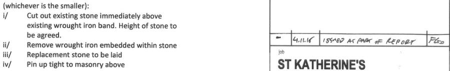
The Following sequence is to be carried out one stone at a time or in max 300mm wide sections
