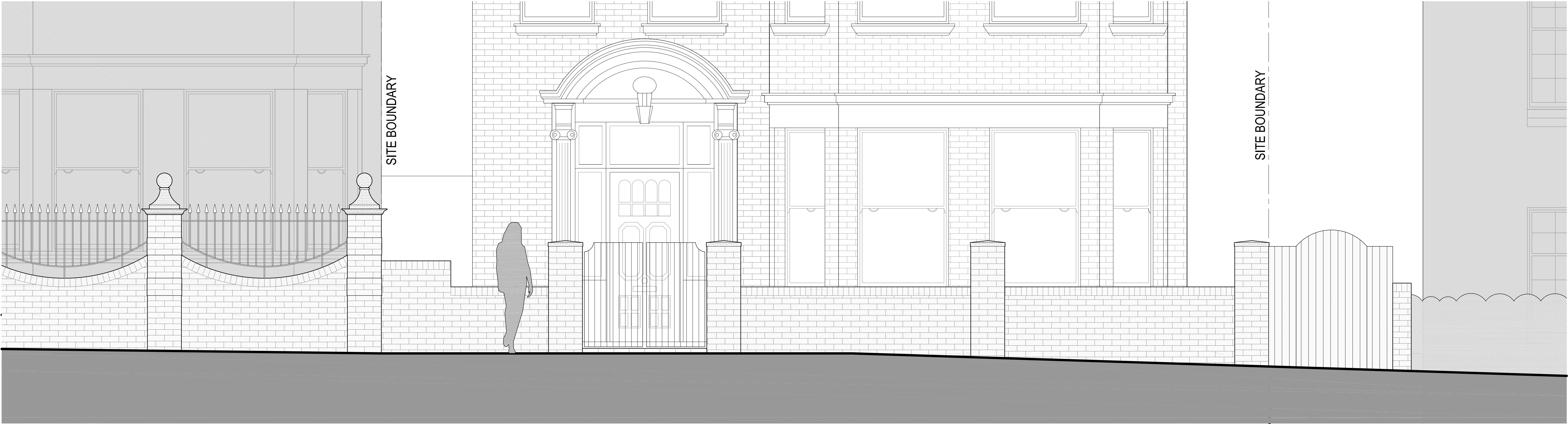
Existing Boundary Wall Elevation Scale 1:25
