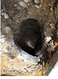
D. Soft low strength brown gravelly sandy CLAY. Gravel consists of brick, concrete, flint, ash and plastic.
