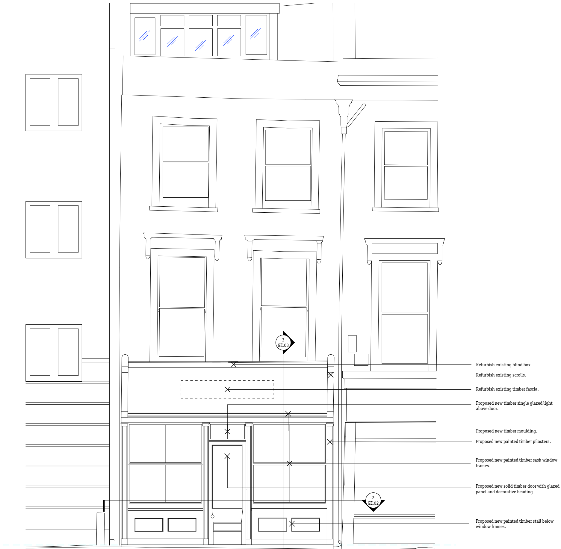
1 Proposed Shop Front Elevation 1:50@A3
