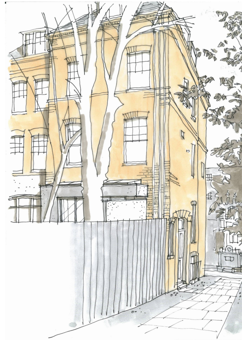
View of rear of property as proposed from Well Walk Passage Showing new bay window & screen wall
