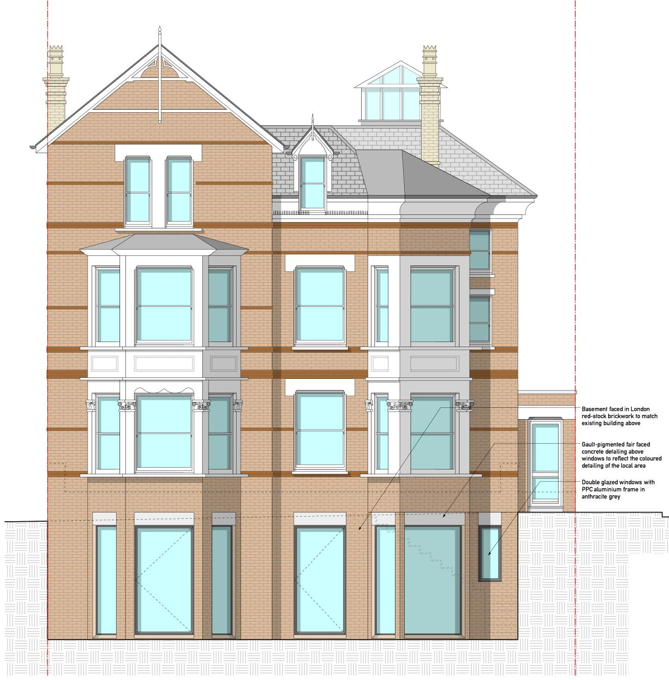
Proposed Front Elevation - Street View Scale: 1:50
