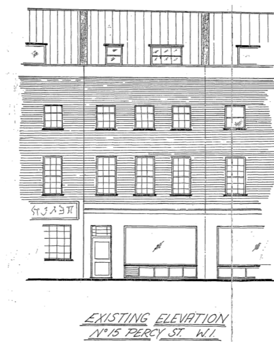
Figure 3: Existing shop front in 1984 fully glazed with a single stall riser
