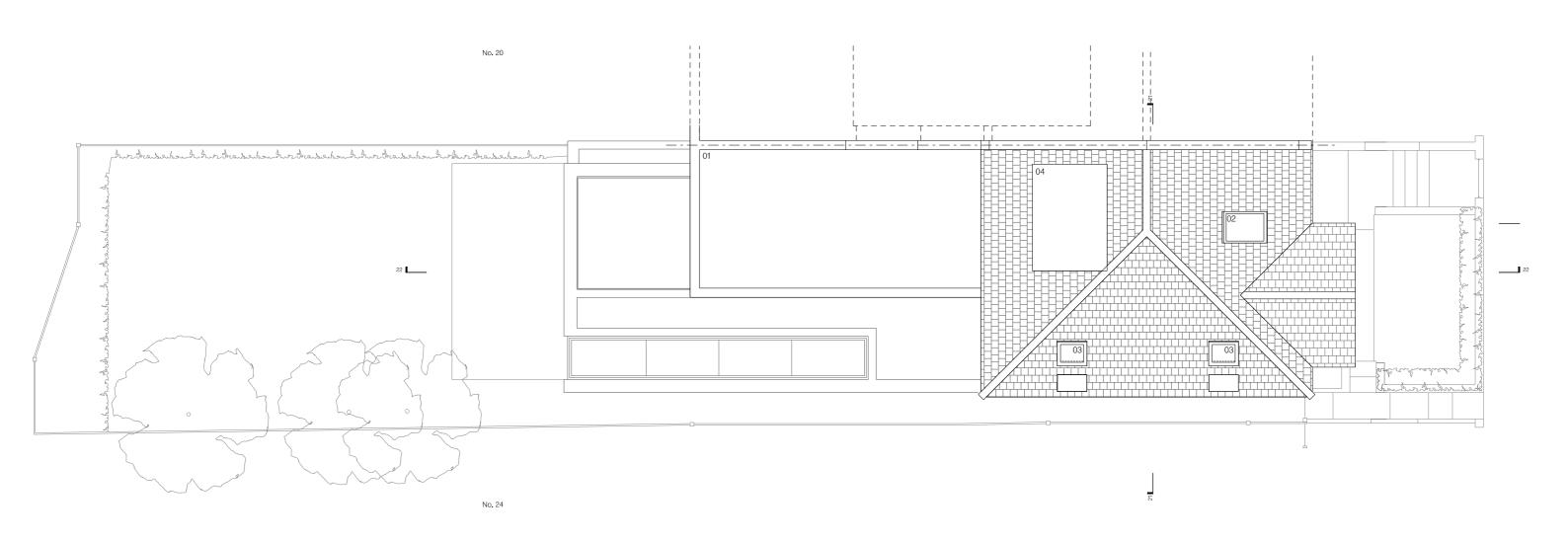
01 LINE OF EXISTING FLAT ROOF BELOW 02 EXISTING ROOFLIGHT 03 NEW PITCHED ROOFLIGHT 04 EXISTING DORMER
