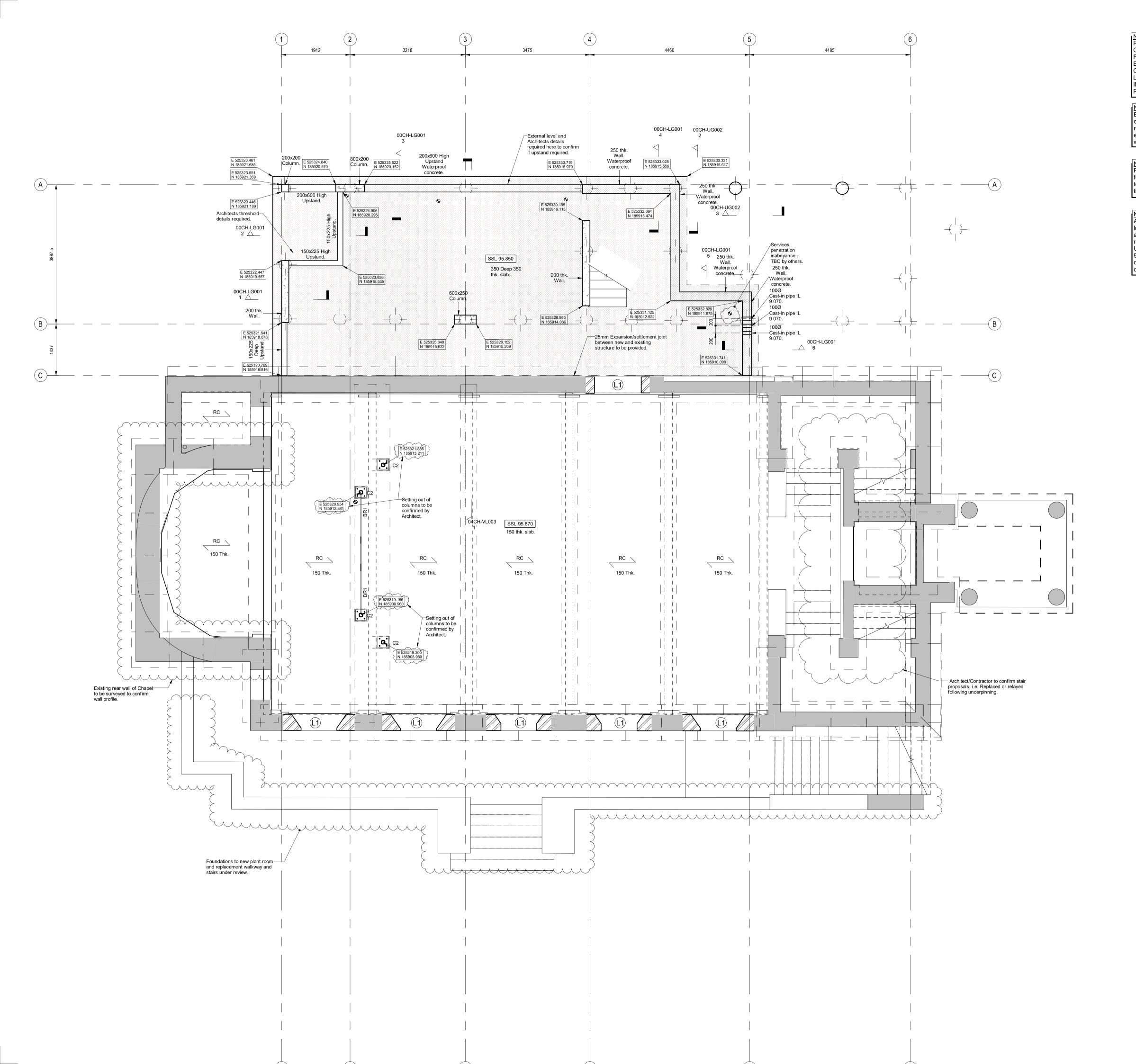
NOTE PROVISIONAL REPAIR ALLOWANCES SHOWN ON THIS DRAWING WILL BE CONFIRMED FOLLOWING REMOVAL OF RENDERED EXTERNAL WALL FINISHES AT EXISTING CRACK LOCATIONS AND INTERNAL DRY LINING. ENGINEER TO INSPECT EACH FLOOR IN TURN AND CONFIRM EXTENT OF REPAIRS REQUIRED.
