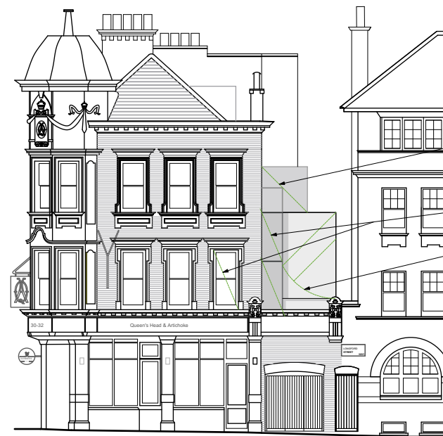
minimal framed glass panels minimal framed side hung glass door dark grey metal panelled lift shaft beyond
