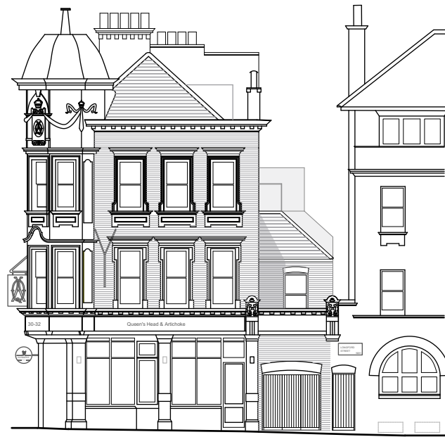
single storey brickwork timber sliding sash window hipped pitched tiled roof
