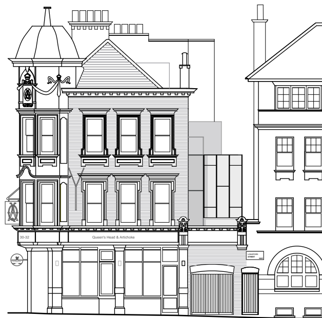
vertical standing seam zinc wall cladding
