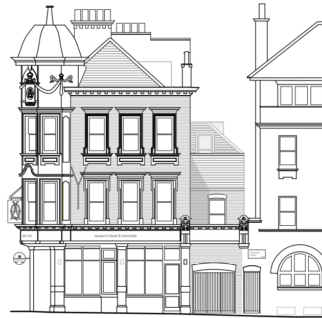
single storey brickwork timber sliding sash window monopitch tiled roof hipped tiled roof to lift beyond with dormer extensions
