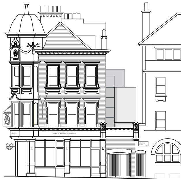
minimal framed glass panels minimal framed side hung glass door with additional glazing bars dark grey metal panelled lift shaft beyond
