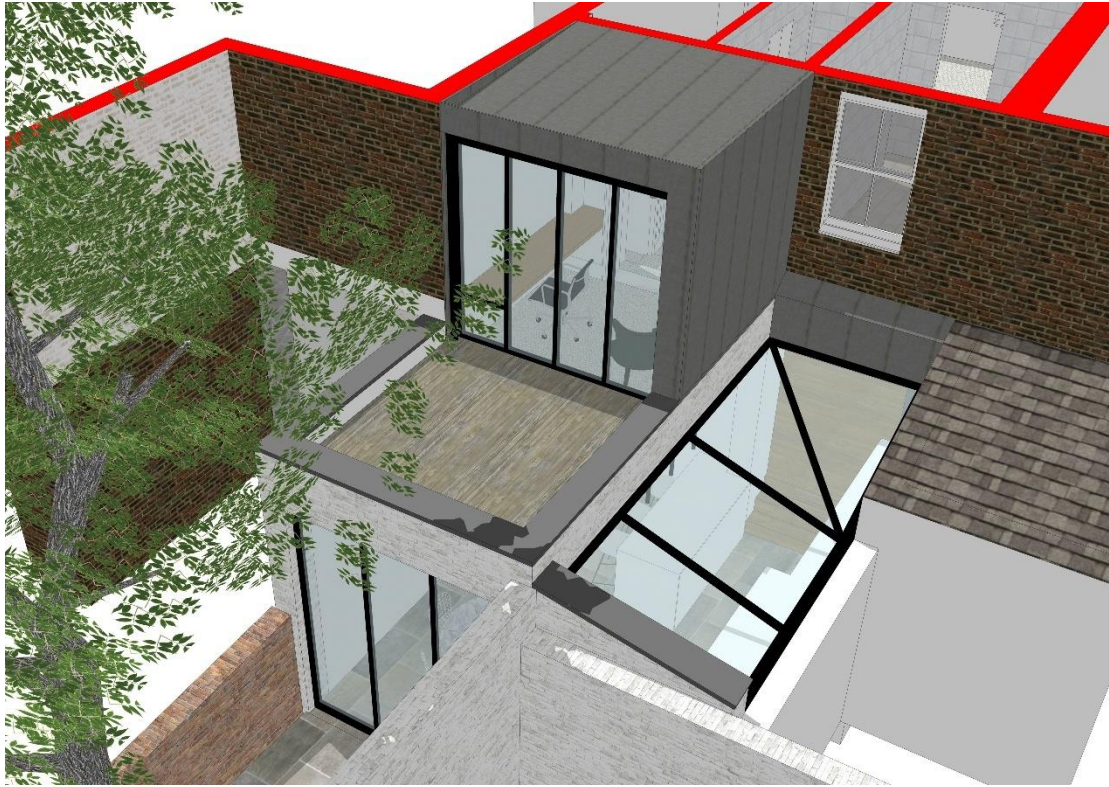
Design concept image showing semi-aerial view of proposed infill glazing and first floor metal clad extension, aligned with rear building line to adjoining lower terrace
