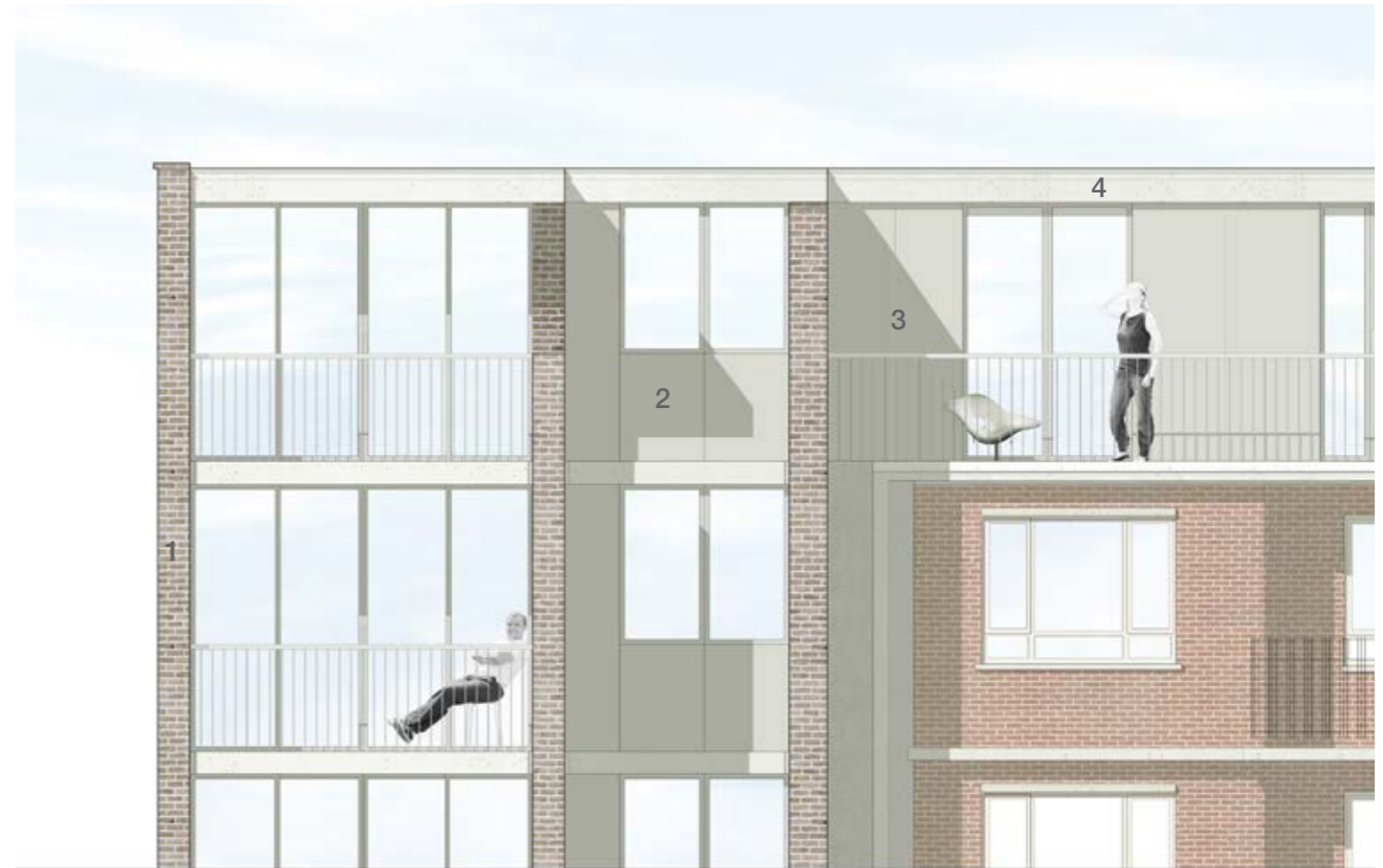
Typical elevation where the side extension connects to the roof extension.
