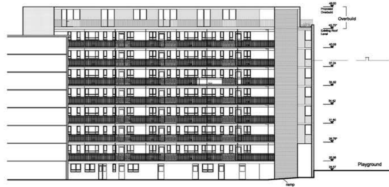
East rear elevation showing extension and changes to existing cladding
