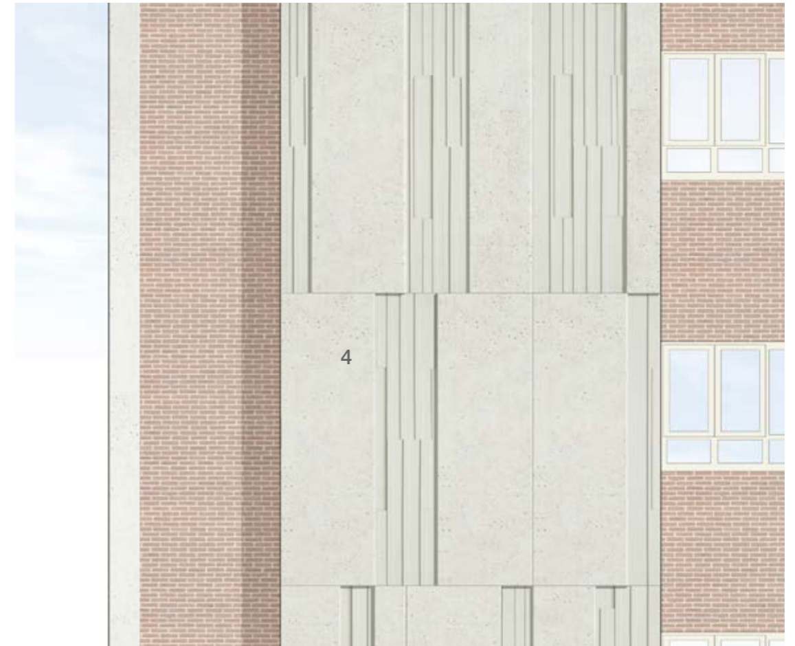
Elevation showing the pre-cast reconstituted stone wall on the north-east elevation of Blemundsby. This sample shows an example of how a texture can be applied to the panels. This can be subject to design development in collaboration with local artists.
