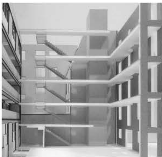
Physical models were used to test the stair & reconciles the complex level differences between existing & proposed in an ordered & logical manner
