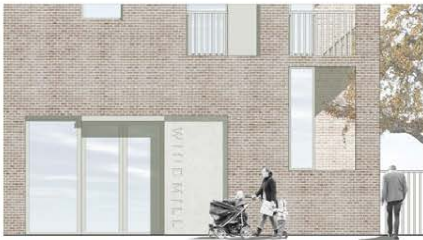
Detailed elevation showing the new main entrance into a new secure lobby. The building is signposted with the block name inscribed in a pre-cast stone panel next to the entrance
