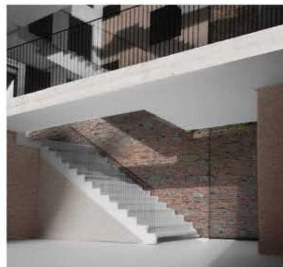
Physical model exploring the junction of the ground floor brick walls with the precast concrete stair, creating a special condition at ground floor & ties the structure into the existing brick walls & garden wall concept
