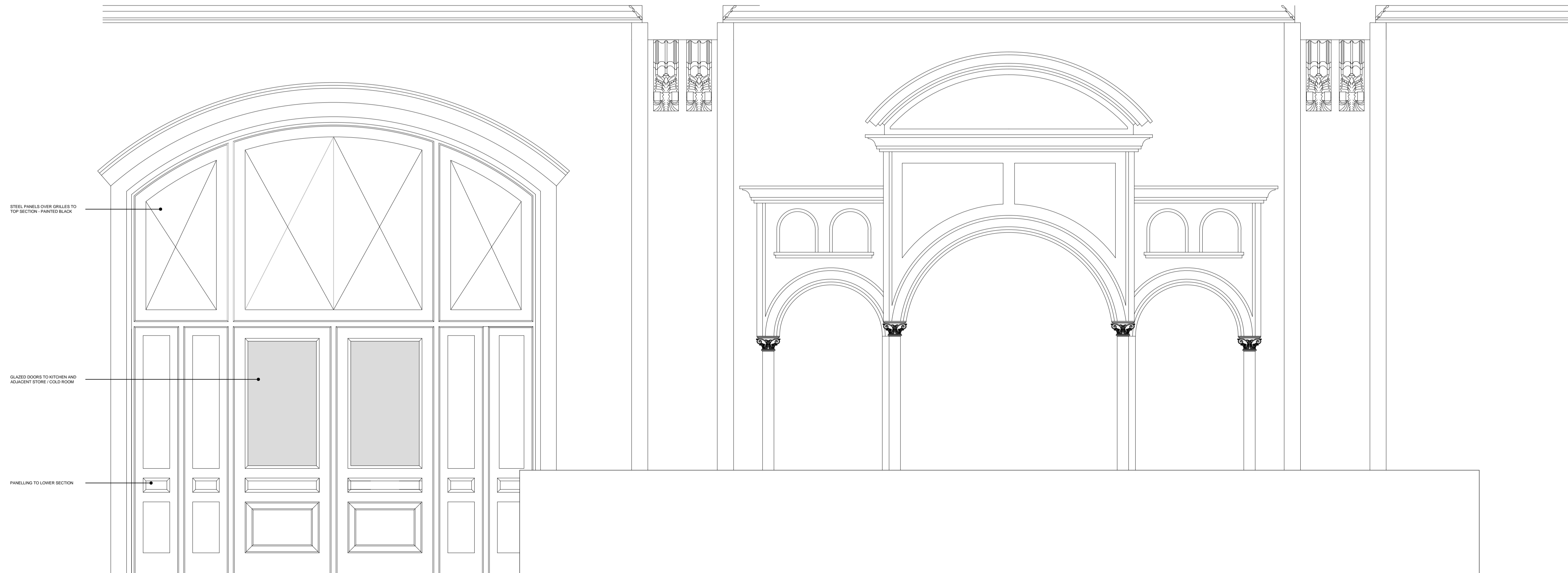
DOOR AND FRAME ELEVATION AS EXISTING Scale 1:20
