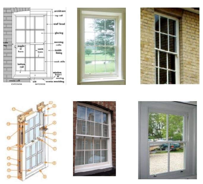
Below, and above right: Proposed timber frame sash window to replace current bathroom window (at rear). the design would either slide vertically, or to open outwards with a latch.
