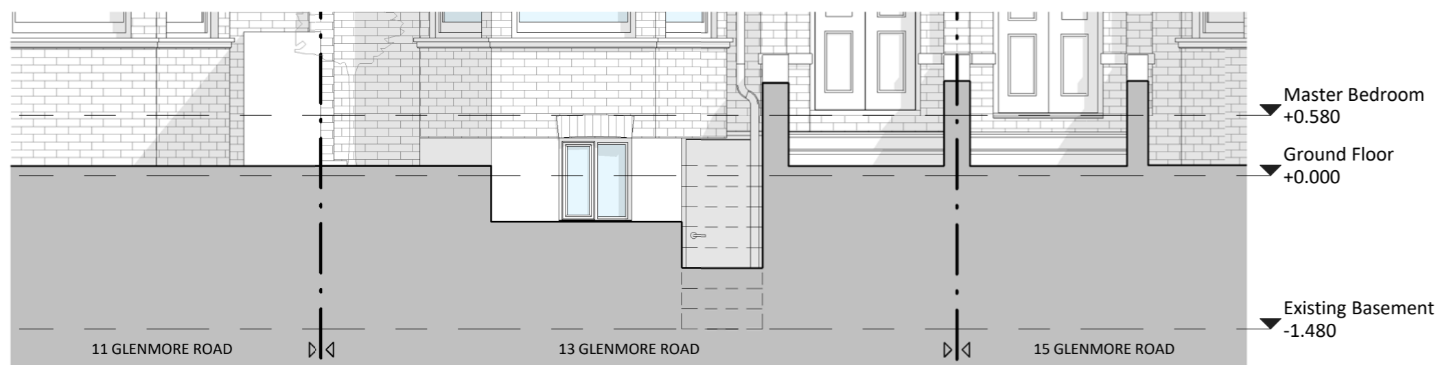
2 Existing North Elevation (Lightwell) 1 : 50
