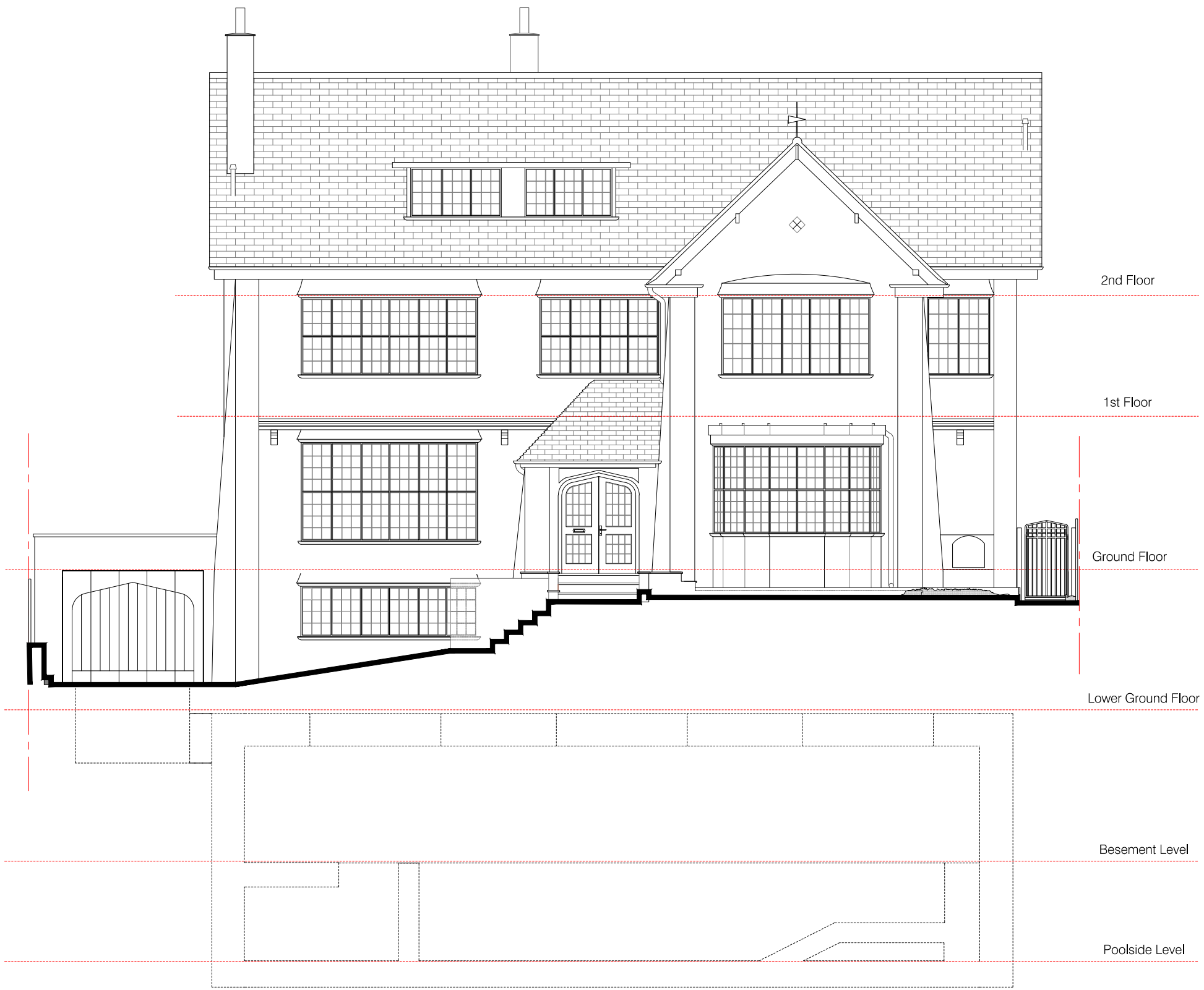
FRONT SECTION A-A' - AS BUILT
