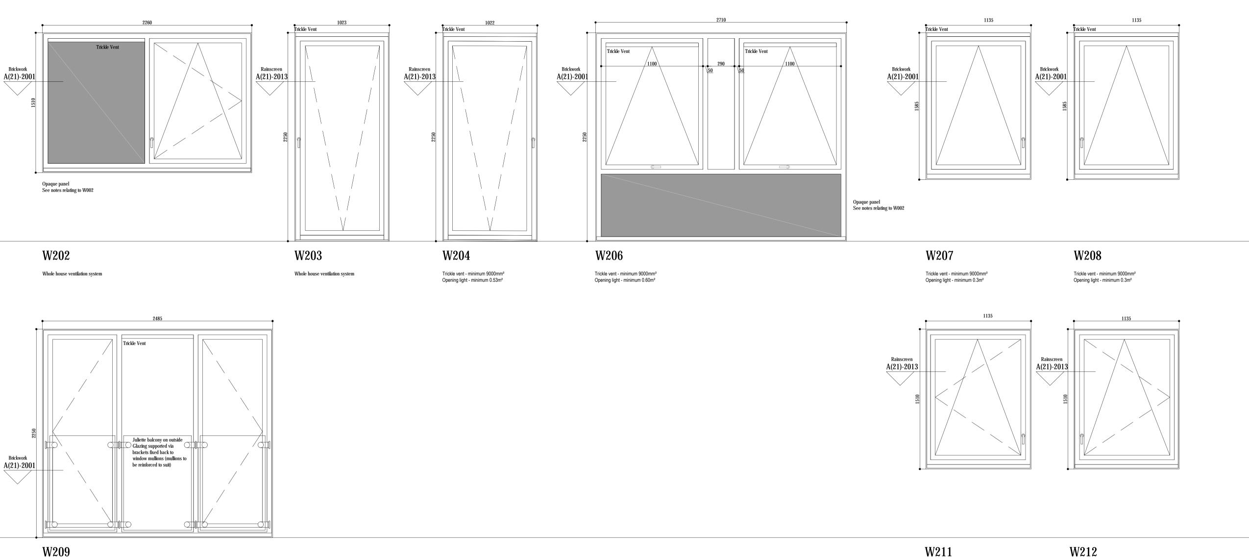
W209 Trickle vent - minimum 20000mm² Opening light - minimum 1.70m²
