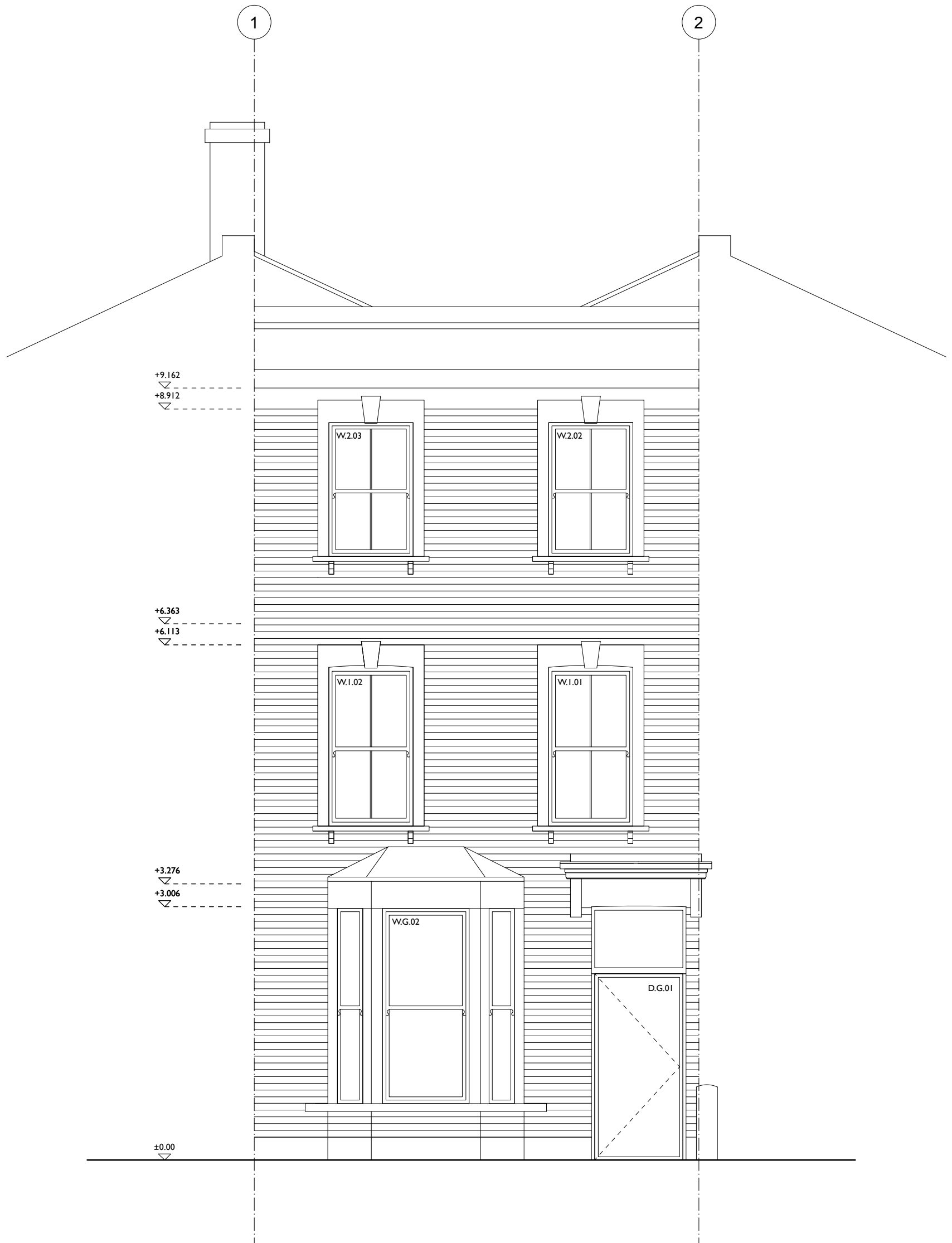
Existing Front Elevation
