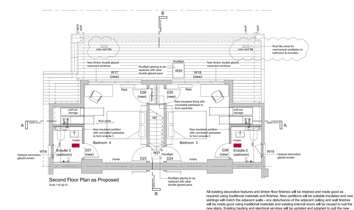
ROOF VENT TILES INDICATED TO ADDRESS PLANNING COMMENTS. DOORS D23 & D24 SWING CORRECTED AND UPDATED FOR TENDER ISSUE. 1. All sizes to be taken and checked on site by the contractor absolute detail prior to preparation of shop drawings or fabrication of parts.
