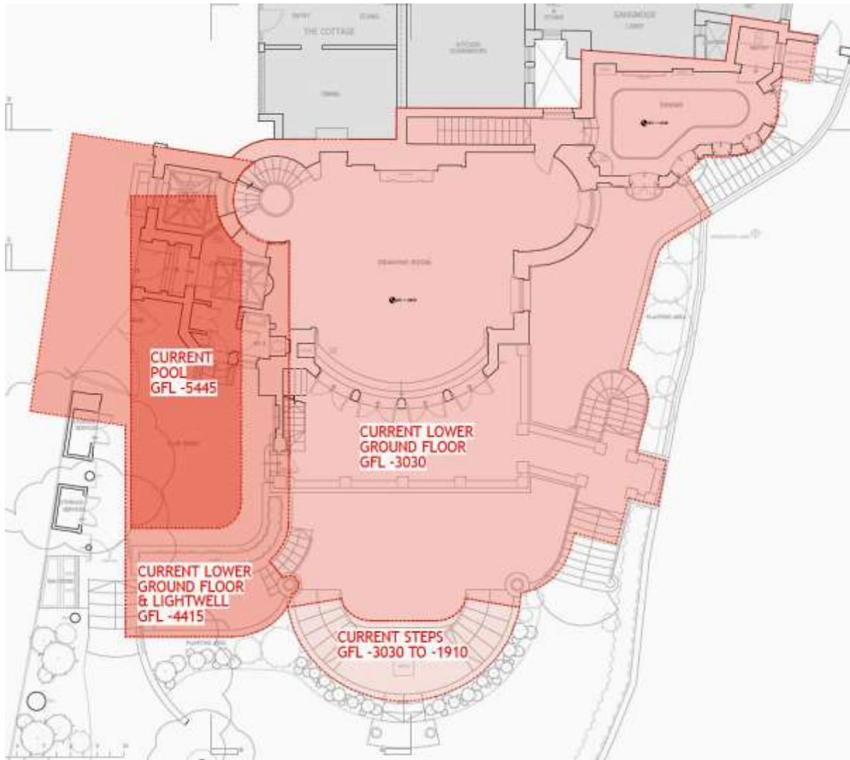
Fig.30: The extent of the current lower ground floor footprint and pool (shown in pink/ red) and including the 2003 additions. Plan provided by Jonathan Freegard Architects (Drawing No. 643-101 current house).
