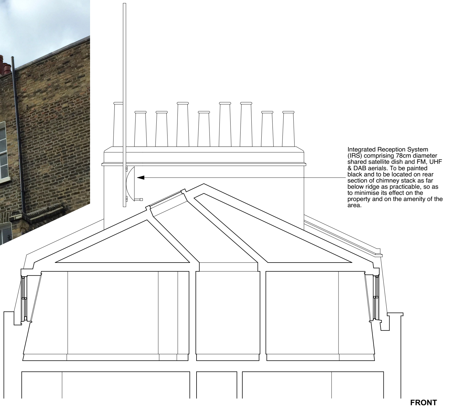
EXAMPLE OF IRS INSTALLATION - SATELLITE DISH (PAINTED BLACK), TV & RADIO AERIALS (at 33 FREDERICK STREET)
