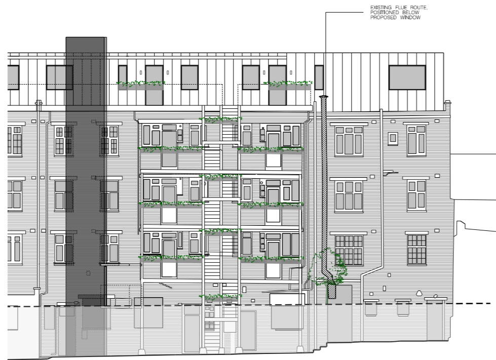
PROPOSED REAR ELEVATION, WITH EXISTING FLUE ROUTE
