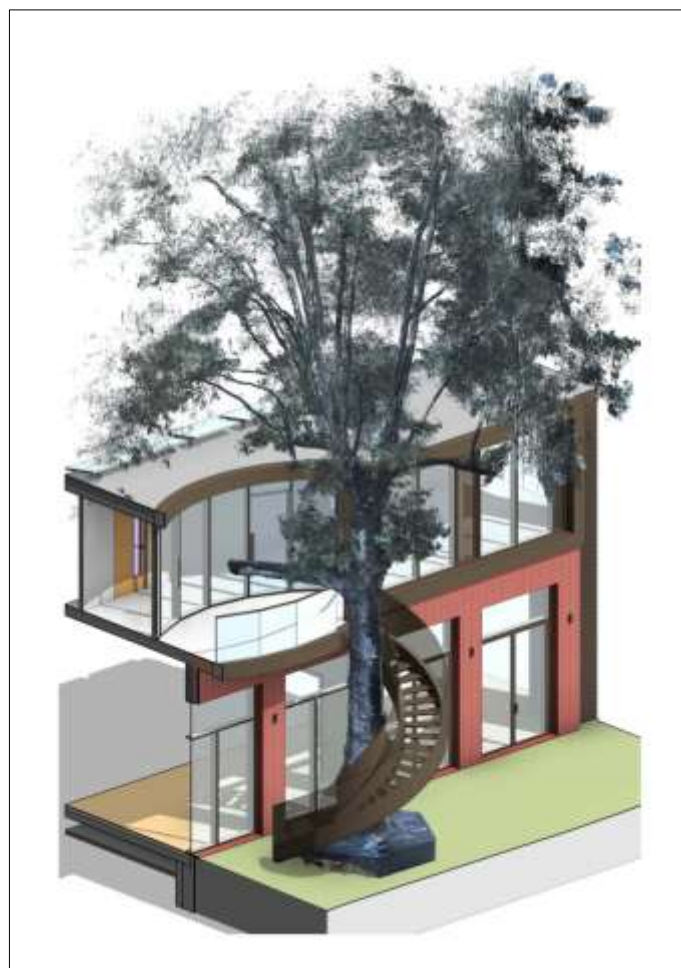
Image 4: Computer 3D model showing that the lowest branch can be cut back to provide space for the classrooms without adversely affecting the shape or health of the tree
