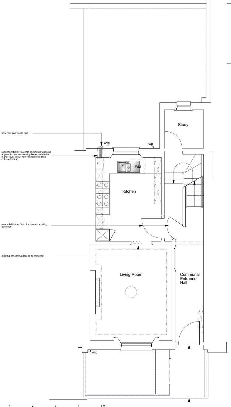
**CONSTRUCTION KEY** existing retained line over/under/behind demolished new construction 28mm thick drylining (incorporating Newton 503 mesh & 12.5mm plasterboard)
