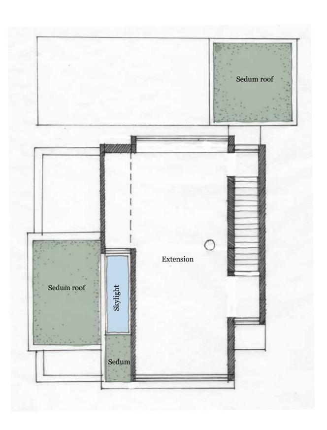
PROPOSED SECOND FLOOR PLAN SCALE 1: 100 at A3 and 1:50 at A1
