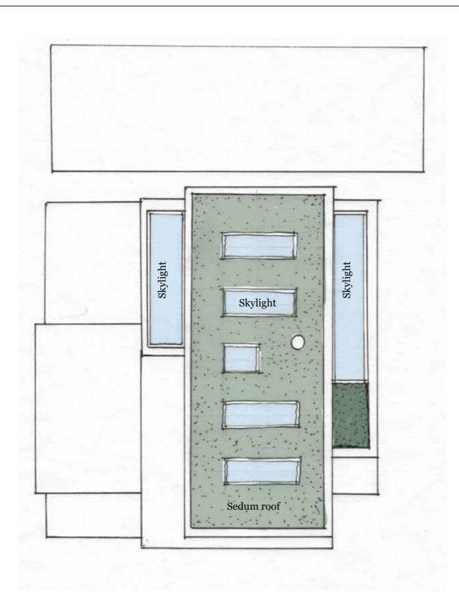
PROPOSED ROOF PLAN SCALE 1: 100 at A3 and 1:50 at A1
