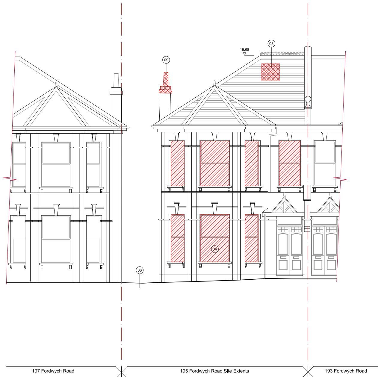
01 DEMOLITION SOUTH WEST (FRONT) ELEVATION A55 SCALE AT 1:100
