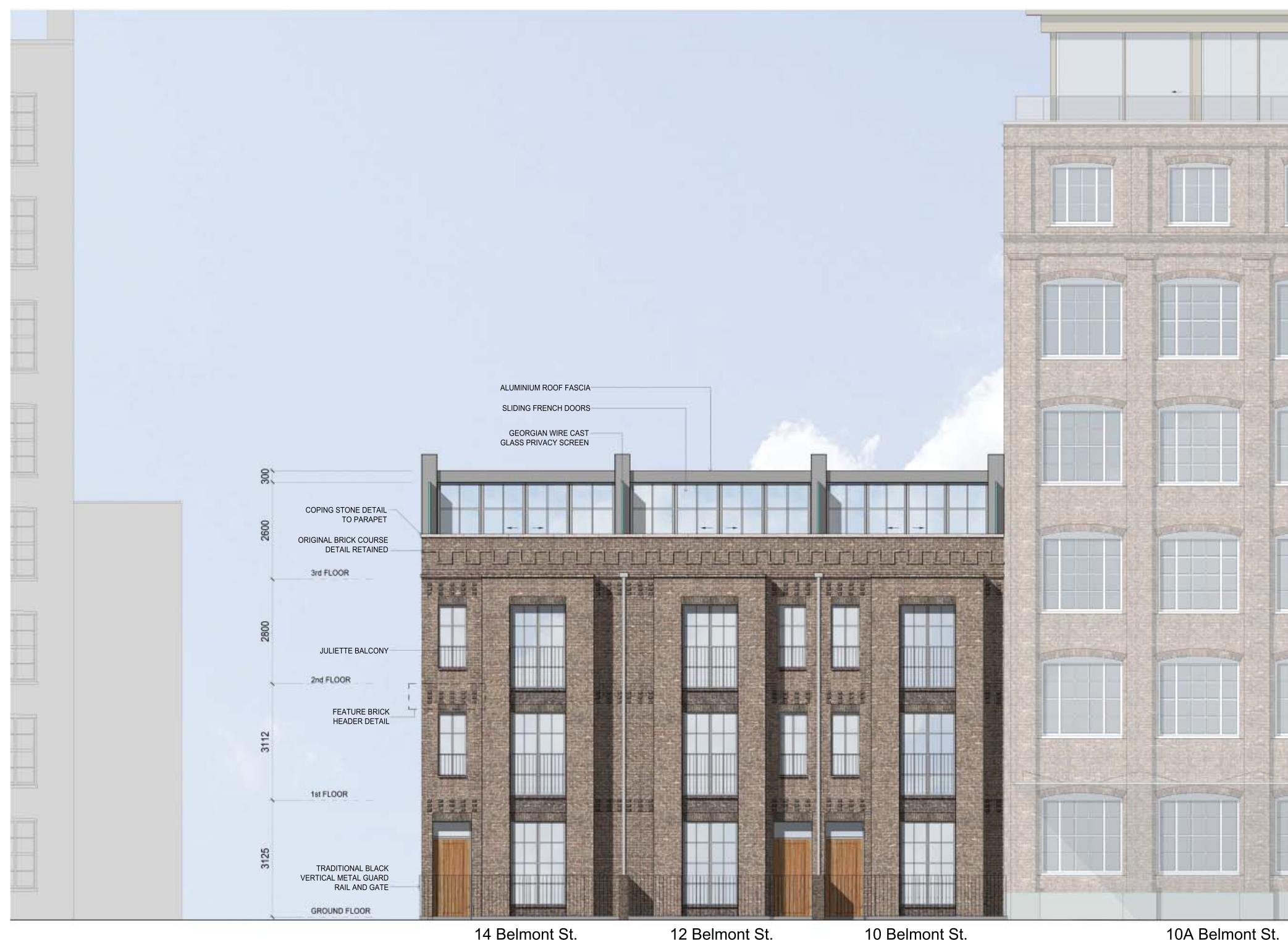
Proposed 10 - 14 Belmont Street west elevation with current approved elevation of 10A Belmont Street
