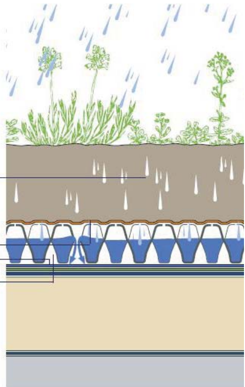
Fig 9: How a green roof releases moisture
