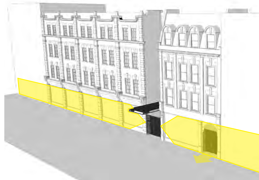
PROPOSED New canopy that extends over Parkway provides a focus on the office entrance, while moving escape alley gates forward to facade line removes ability for vagrancy
